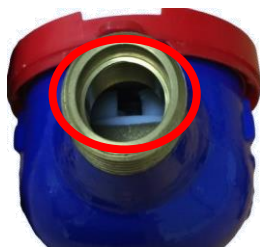
Check the condition of the outlet section to see if it is clean and there is no dirt/object stuck on the measuring chamber.
