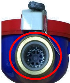
Check the condition of the filter at the inlet section to see if it is still intact and clean
